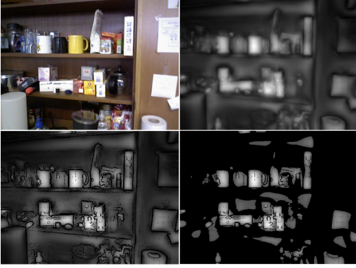
Figure 2: Top left to bottom right: original RGB image; its corresponding saliency map SM ; saliency map after adaptive thresholding SM' ; the SM'' map after the final thresholding.
