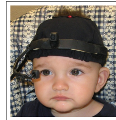
Figure 4: Snapshot of an infant (at 6 months) with a head-mounted eye-tracking device.
